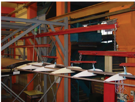
Fig. 24 Mechanical equipment for shear, bending, and torsion test on HeliPlat scaled-size prototype.
